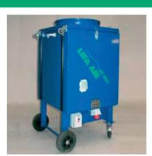
Lifa AirClean 8000 is a multi-function machine. Its main use is for creating negative pressure and cleaning large and broad ventilation duct systems. The vacuuming unit is able to create not only a large air volume, but also a "gale force" airflow of 18-22m/s which ensures the total removal of brushed dirt.
